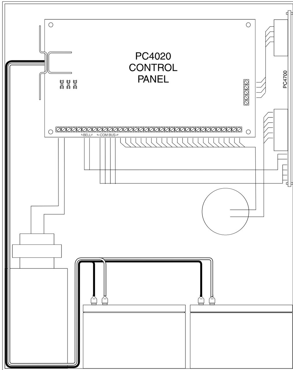
**INSTALL BATTERY AND AC WIRING
