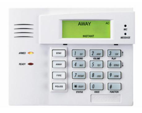
The keypads contain a built-in loudspeaker (sounder) that will annunciate during alarms and troubles. The keypads also beep during certain system functions, such as during entry/exit delay times, in CHIME mode, and when you depress any of the keys (to acknowledge the key press).
